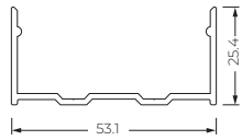
Aluminium Mounting clips 20x53.1x25.4mm(L x W x H) Accessories: Screw M3X16mm
